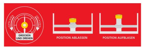
Now connect the hose of the pump to the valve and pump up the three chambers of the kayak one after the other to a pressure of 0.7 bar.
