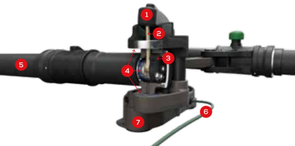
1. Powerful rocker arm / 2. High strength con rods with ball heads / 3. Positioning cam for defined blade positions / 4. Smooth running ball bearings for easy oar blade feathering / 5. Carbon fibre tubes for handle and oar blade / 6. Release leash to fold up the sculls / 7. high strength pivot rowlock
